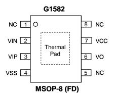
Note: Recommend connecting the Thermal Pad to the Pin#4 VSS for excellent power dissipation.
