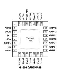
Note: Recommend connecting the Thermal Pad to the Ground for excellent power dissipation.
