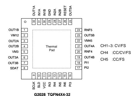
Note: Recommend connecting the Thermal Pad to the Ground for excellent power dissipation.
