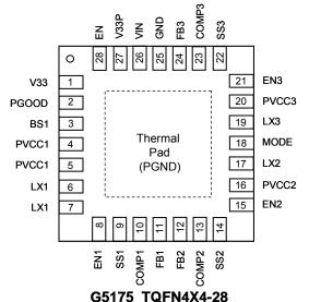
Note: Recommend connecting the Thermal Pad to the round for excellent power dissipation.
