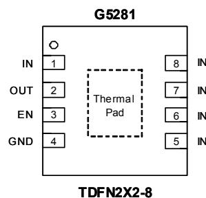
Note: Recommend connecting the Thermal Pad to the GND for excellent power dissipation.
