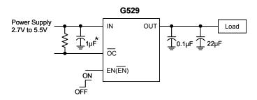
\*: 1µF of input capacitor is enough in most application cases. If the PCB trace of power rail to IN is long, larger input capacitor is necessary.
