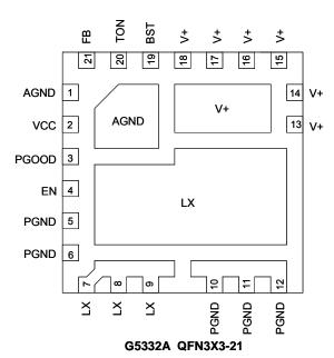
Note: Recommend connecting the Thermal Pad to the Ground for excellent power dissipation.
