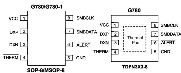
Note: Recommend connecting the Thermal Pad to the GND or let it keep floating.
