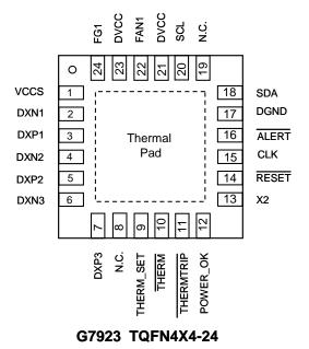
Note: Recommend connecting the Thermal Pad to the Ground for excellent power dissipation.
