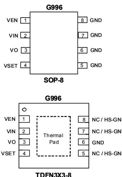
Note: Recommend connecting the Thermal Pad & 5,7,8 to the GND for power dissipation.
